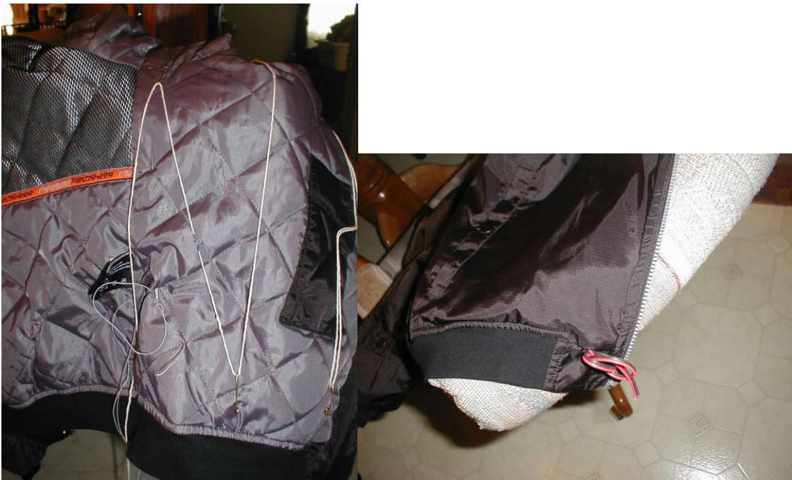
Photograph: left – 30 AWG on needle following string line guide Photograph: right – 18 AWG pigtail connected to both ends of 30 AWG (starting point/ending point)
