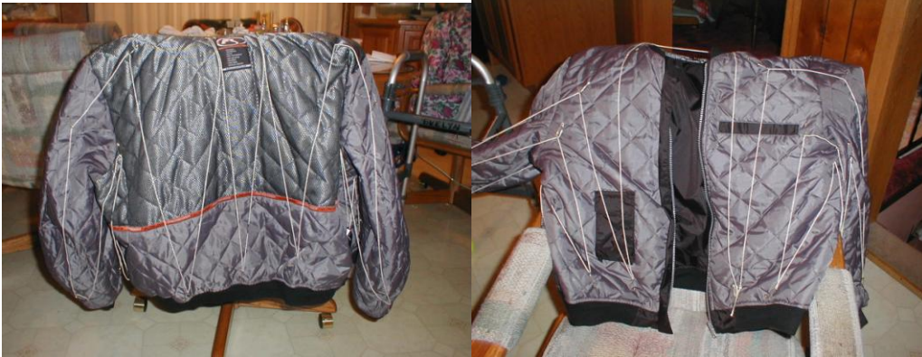
Photographs: left and right – String line guide layout on back and front of liner (inside out)
